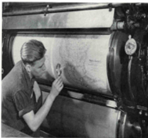
Locked on the Big Rotary Presses, the Plates Are Ready to Start Rolling
